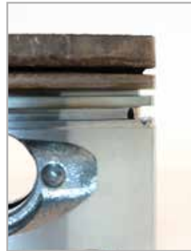
Piston with dirty piston ring grooves.
